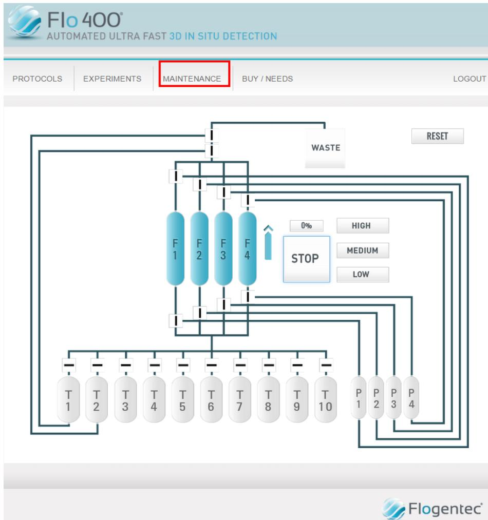
You can test the device and change connections between tankers and Flowcells thanks to square connection
